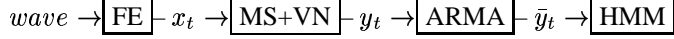
Figure 1: Block diagram of our feature processing method. FE: feature extraction, MS: mean subtraction, VN: variance normalization, ARMA: smoothing filter, HMM: ASR training and decoding
