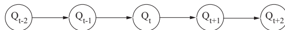
Figure 13: A simple first order Markov chain. This graph encodes the relationship Q_t \perp\!\!\!\perp Q_{1:t-2} | Q_{t-1} .
