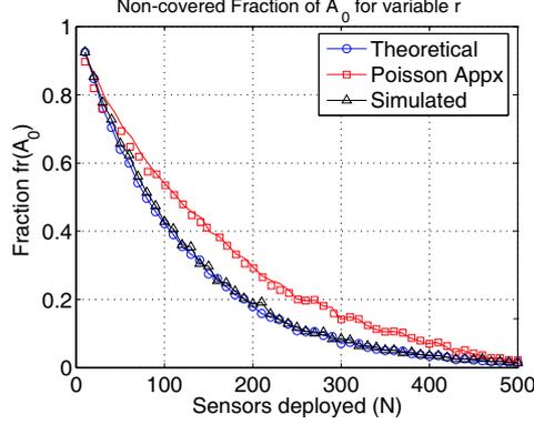
Fig. 9. Fraction  $fr(\mathcal{A}_0)$  of  $\mathcal{A}_0$ , that remains non-covered as a function of the number of sensors  $N$  that are deployed to monitor the  $FoI$ , for the heterogeneous network deployed in the second experiment.
