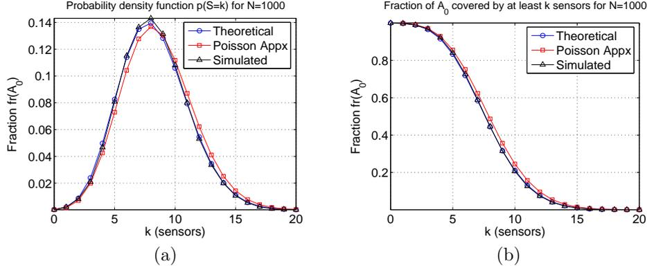
Fig. 7. (a) The pdf of the fraction  $fr(\mathcal{A}_0)$  covered by exactly  $k$  sensors when  $N = 1000$  sensors with identical sensing area are randomly deployed. (b) The fraction  $fr(\mathcal{A}_0)$  covered by at least  $k$  sensors when  $N = 1000$  sensors with identical sensing area are randomly deployed.
