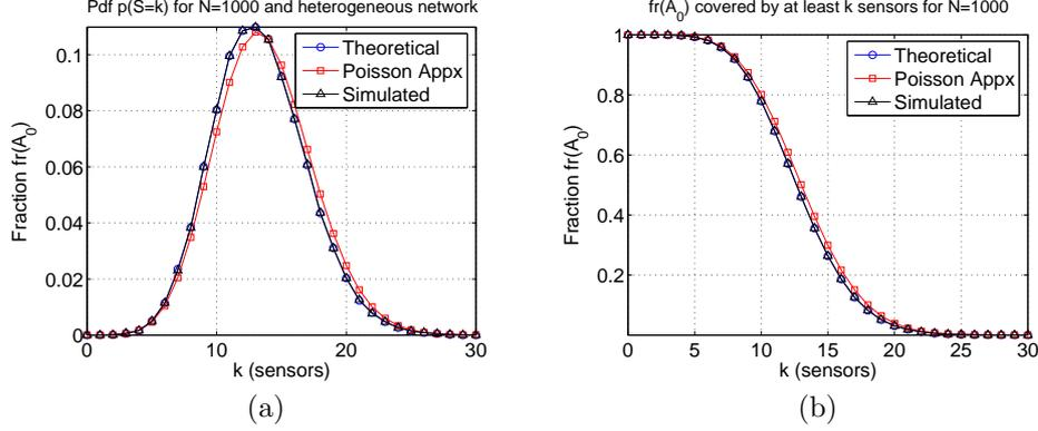
Fig. 11. Heterogeneous sensor network, with  $FoI$  being a disk of radius  $R = 100m$ . An equal number of two types of sensors are deployed; Type  $A$  has a sensing area of a disk shape with radius  $r_A = 10m$ , while type  $B$  has a sensing area of a disk shape with  $r_B = 15m$ . (a) The pdf of the fraction  $fr(\mathcal{A}_0)$  covered by exactly  $k$  sensors when  $N = 1000$  sensors. (b) The fraction  $fr(\mathcal{A}_0)$  covered by at least  $k$  sensors when  $N = 1000$  sensors.
