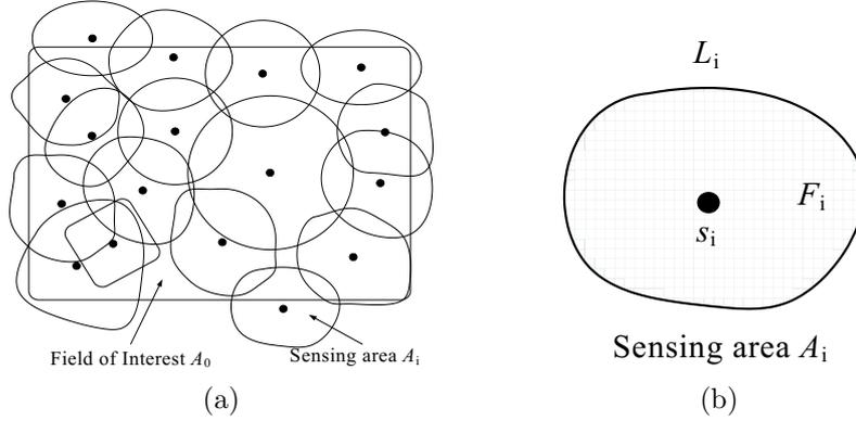
Fig. 2. (a) A heterogeneous sensor network with randomly deployed sensors covering an  $FoI \mathcal{A}_0$ , (b) The sensing area  $\mathcal{A}_i$  of a sensor  $s_i$ .
