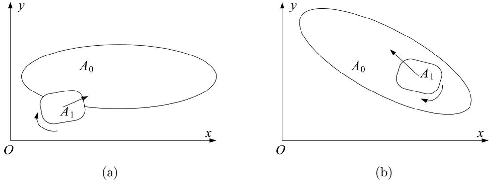
Fig. 3. (a) Set  $\mathcal{A}_1$  is free to move within the plane in such a way that it intersects with fixed set  $\mathcal{A}_0$ . (b) Fixed set  $\mathcal{A}_0$  has a different initial orientation and position. The measure of the set of positions of  $\mathcal{A}_1$  such that it intersects  $\mathcal{A}_0$ , expressed via the kinematic density, is the same regardless of the initial configuration of the two sets. The measure is invariant to translations and rotations of any of the two sets.
