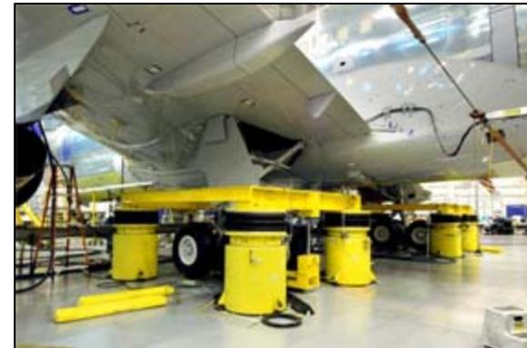
Ground Vibration Testing Advancements BCA & IDS platforms
