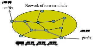
At an **intermediate** level the achievable long-term performance of the roro-terminal was investigated. Presupposing a roro-terminal with three independent rails and a frequency of one train every 40 minutes per rail we achieve a throughput of more than 2000 articulated vehicles per day. These results are achieved with very few resources, e.g. a parking area for the transient vehicles of less than 200 places, even for statistically distributed traffic volumes with high variance.
