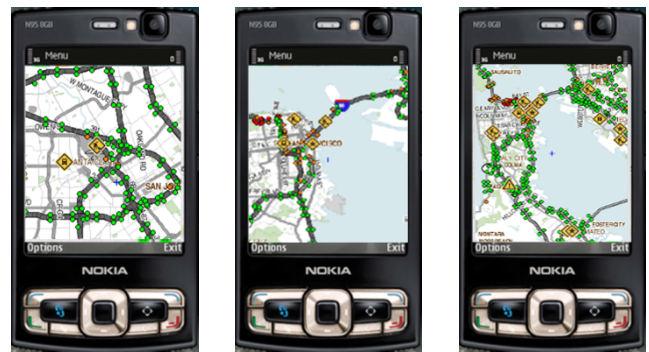
Fig. 1. Mobile Millennium traffic client. Traffic is displayed directly on the phone screen, with traffic information (construction, accidents, etc.), and audio traffic reports. For drivers who want to opt in, the phone can also send information to the system (Lagrangian measurements).
