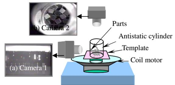
Fig. 2: Experimental set-up for parts assembly: The template is attached to a coil motor whose vibration is controlled by a function generator and optional power amplifier. The parts are confined to a volume above the template using an antistatic cylinder.
