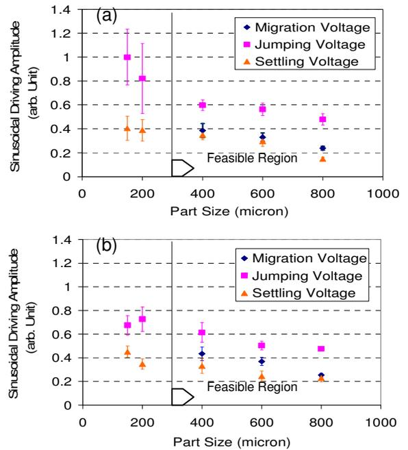
**Fig. 4:** Migration Voltage, Jumping Voltage and Settling Voltage for different part sizes from 150 $\mu\text{m}$  to 800 $\mu\text{m}$  scaled to the highest average value. Graph (a) is for double side polished parts on smooth surface and (b) double side polished parts on rough surface. The vertical bar shows the standard deviation of experimental results from five different measurements.
