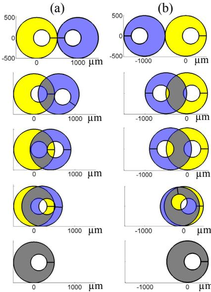
Figure 5. Dynamic simulation snapshots: With the initial position (dark/blue) of the part at either side of the binding site (light/yellow), the part aligns with the binding site due to continuous surface tension force.
