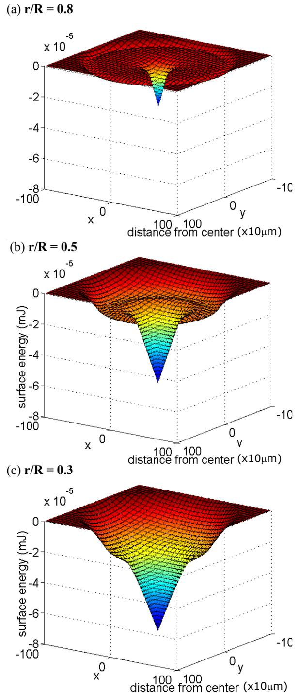
Figure 2. Translation energy profiles show surface energy as a function of relative part position for rings with different cutout ratios  $r/R$ . Energy is minimized with exact alignment. Other local minima exist for (a)  $r/R = 0.8$  and (b)  $r/R = 0.5$ , but not for (c)  $r/R = 0.3$ .
