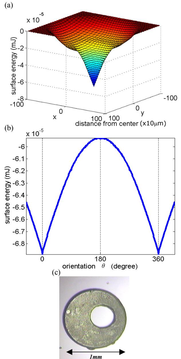
Figure 4. Energy profiles for offset ring design with  $(R, r/R, d/R) = (500\mu\text{m}, 0.4, 0.24)$ . (a) A global minimum of surface energy is found at  $(x,y)=(0,0)$  while translating the part over the binding site. (b) The global minimum also appears when part orients with the binding site for  $(x,y)=(0,0)$ . (c) Experimental result shows exact alignment of the silicon part over the SAM-coated gold binding site in water.
