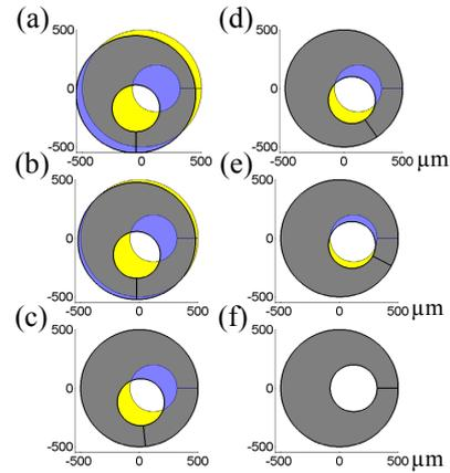
Figure 7. Dynamic simulation with initial placement set as  $(x, y, \theta) = (-50, -50, 270^\circ) \rightarrow (0, 0, 0^\circ)$ . Translation of the part takes place before rotation begins.
