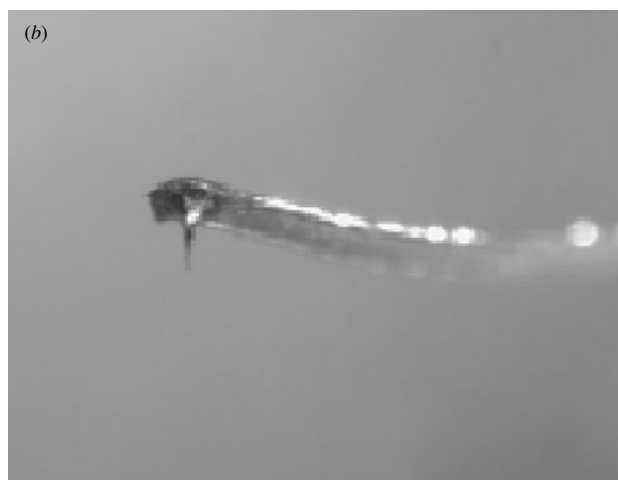
Figure 9. (a) Released devices with PI support. (b) A needle with PI support. This device was produced using a single pillar protected by narrow side walls.
