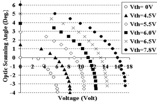
Figure 5: The switch characteristics under the dual-servo-scanning mode ( $V_{th}$  = thermal voltage)
