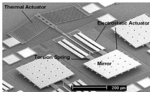
Figure 1: The dual-servo mirror
