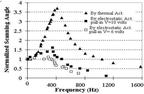
Figure 4: Frequency response by using the thermal and electrostatic actuator to drive the mirror. The measured natural frequency is 416Hz. The electrostatic actuator with lower pull-in voltage shows more squeeze film damping.
