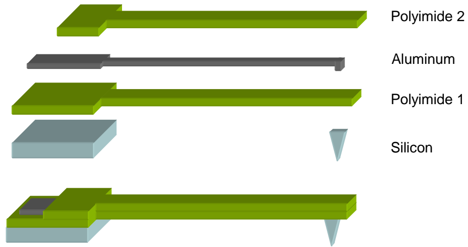
Figure 3.8: Schematic of the flexible neural implant device
