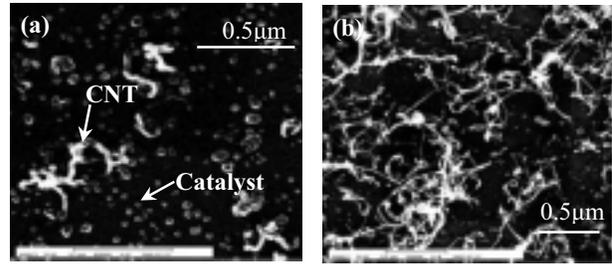
Figure 3: SEM images of CNT with different water vapor concentrations in deposition. (a) 600ppm. (b) 721ppm.
