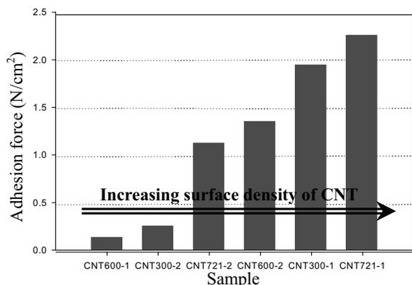
Figure 8: Measured adhesion force of CNT.
