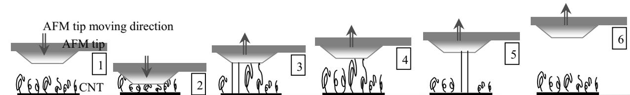
Figure 6: Stretching mechanisms of CNT during AFM measurement.
