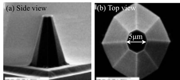
Figure 4: SEM images of the AFM plateau tip.
