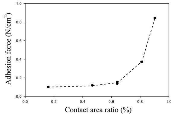
Figure 7: Measured adhesion forces of polymer nano-fibrils as a function of contact area ratio.
