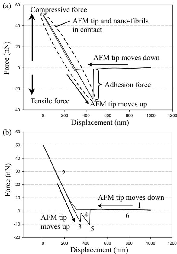
Figure 5: AFM force-displacement measurement of artificial nano-fibrils. (a) ZEP 520A nano-fibrils (100nm width and 100nm spacing). (b) CNT.
