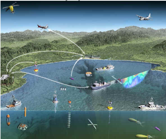
Figure 6: Schematic diagram showing the synergistic integration of in situ and remote sensing sensors in Monterey Bay.
