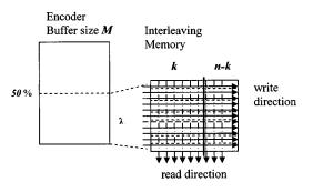
Fig. 3. Block diagram for the combined encoder buffer and the interleaver.
