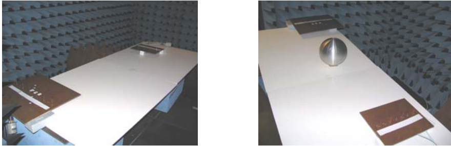
Figure 3. Experimental verifications in the anechoic chamber. Left: free space, Right: around conducting sphere.
