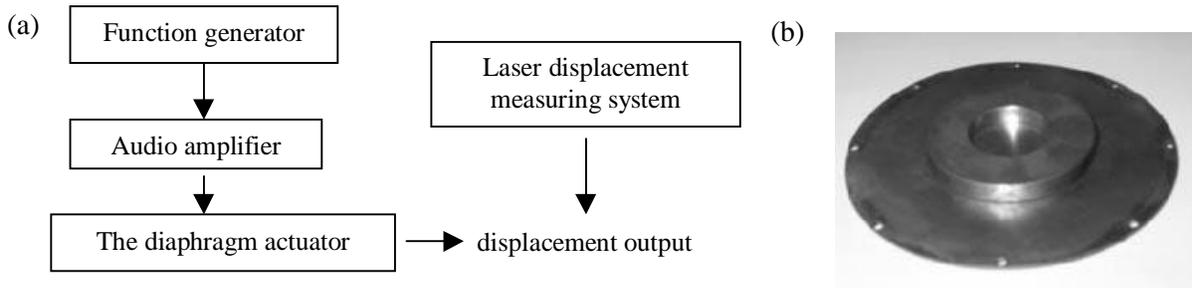
Figure 6 (a) Block diagram of the measurement system for performance tests of the diaphragm actuator, (b) the ferromagnetic shape memory alloy composite diaphragm
