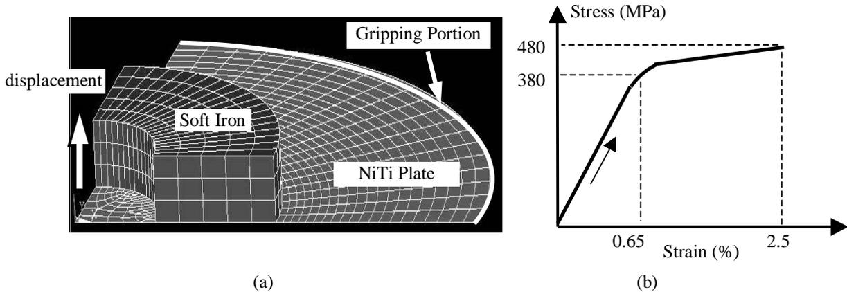
Figure 2 (a) ANSYS model of the quarter composite diaphragm, (b) the nonlinear stress-strain curve of NiTi SMA as input material data.
