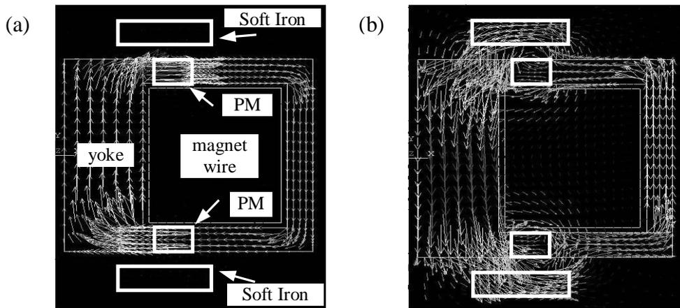
Figure 4 Electromagnetic FEM analysis simulates the function of the hybrid magnet system where PM is the permanent magnet, (a) magnetic flux is flowing inside the yoke and no force is available on soft iron when the power is off, (b) magnetic flux goes through soft iron pad and force is induced when the power is on
