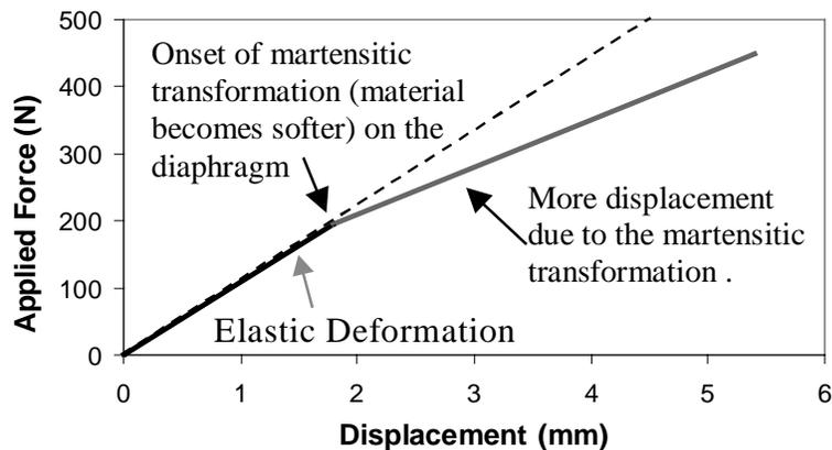
Figure 3 Estimated force-displacement of NiTi/soft iron diaphragm
