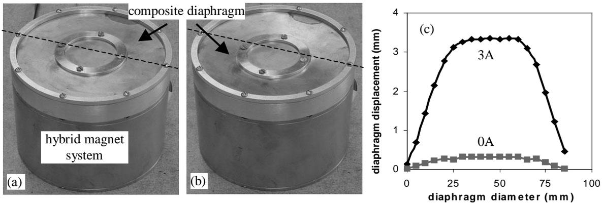
Figure 7 The photos of the diaphragm actuator, (a) power is off, (b) the diaphragm deforms downward when the power is on and (c) The cross section profile along the diameter of the diaphragm without input current (blue line) and with 3Amp current (black line).
