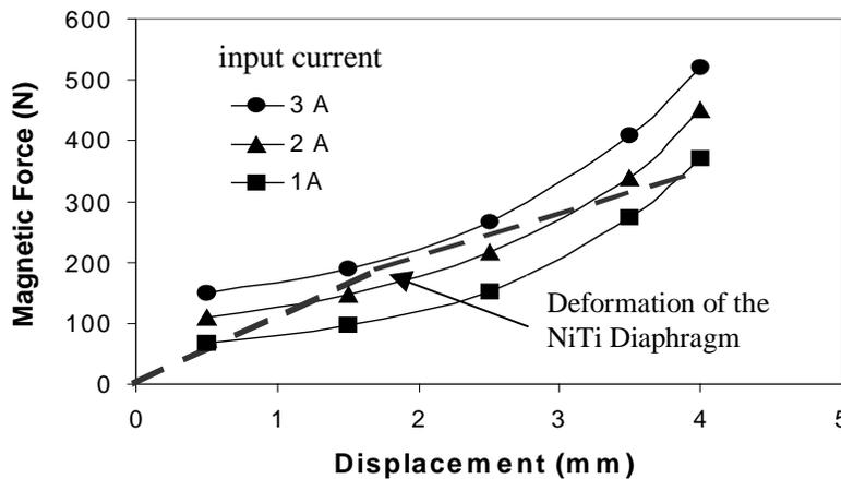
Figure 5 Estimated force-displacement relation of the diaphragm actuator
