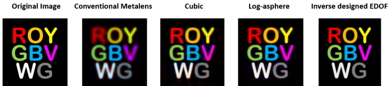
Figure 19. Simulated imaging performance after deconvolution. Deconvolved images captured by the EDOF imaging system, using the simulated images and PSFs.
