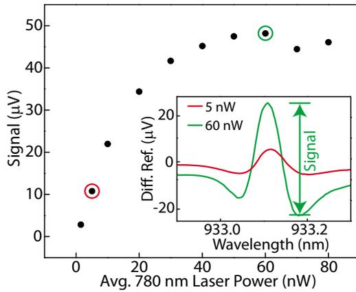
FIG. 3. (Color online) Signal strengths in DR spectra as a function of 780 nm laser power for a QD resonant with a PCC. The tunable cw laser is kept at 20 nW and the 780 nm laser is modulated at 10 kHz. The signal is taken as the difference between maximum and minimum values in each DR spectrum and is shown to saturate at higher powers. Inset: DR spectra for 780 nm laser powers of 5 nW and 60 nW.
