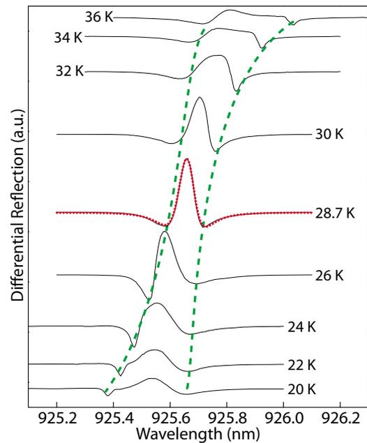
FIG. 2. (Color online) DR spectra (offset) obtained at different sample temperatures with a 6 nW tunable cw laser and a 20 nW 780 nm laser modulated at 20 kHz. Temperature variation serves to tune the QD through the cavity resonance. The dotted curve is a fit of the analytical expression for  $\Delta R$  to the 28.7 K trace. The two dashed lines are guides to the eye to show the anti-crossing of the polariton peaks corresponding roughly to the minimum values in each spectrum.
