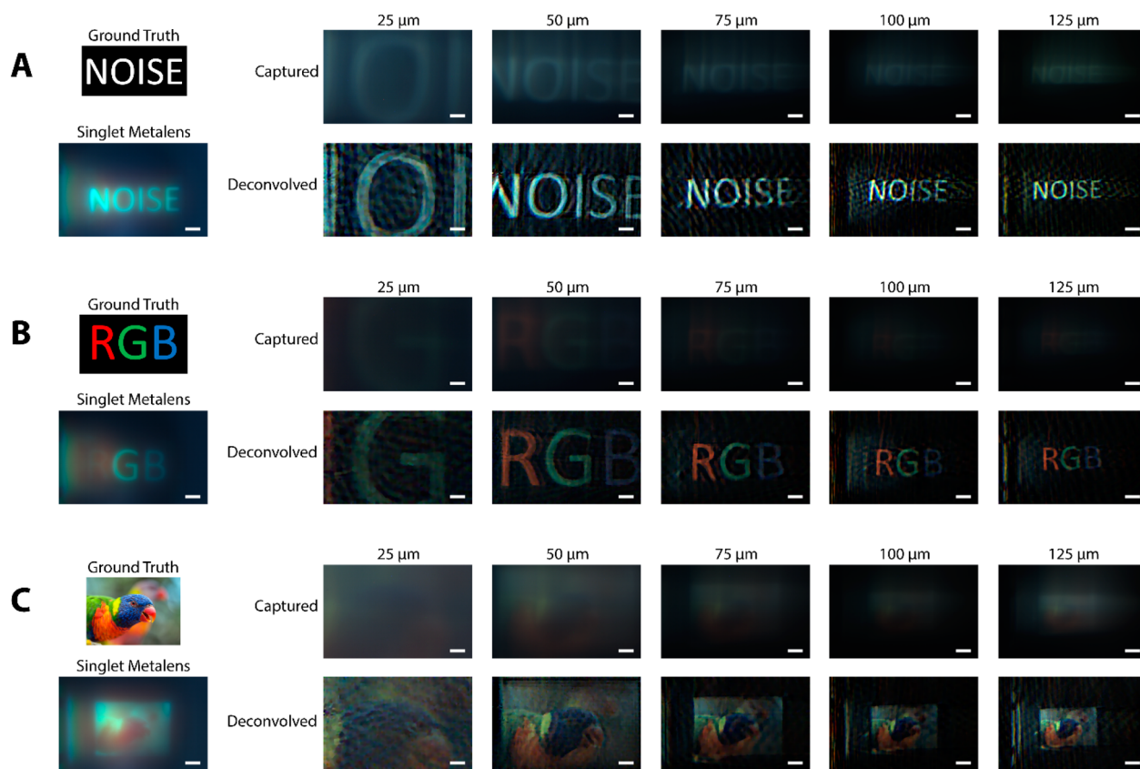
Figure 6. White light imaging. Images are shown depicting the ground truth objects that were imaged, including “NOISE” text (A), “RGB” text (B), and a colorful bird (C). Also shown are images captured using the 1.5 mm singlet metalens under white light for comparison, and the images from the Alvarez EDOF metalens before and after deconvolution for five different lateral displacements ranging from 25 to 125 \mu\text{m} from left to right. Scale bar 62 \mu\text{m} in all images.
