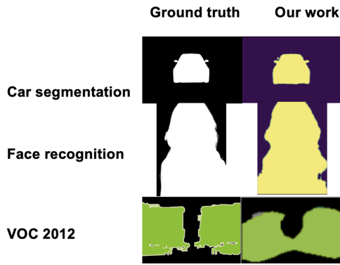
Fig. 6. Examples of object segmentation for the considered benchmarks of (i) car segmentation, (ii) face recognition, and (iii) VOC2012. Left to right: Input image from data sets, ground truth, our work (SCLC/OSCLC).
