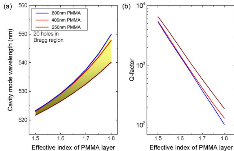
Fig. 4. (a) The plot shows the change in the cavity mode wavelength with the effective index of the PMMA layer for different PMMA layer thicknesses, namely 250 nm, 400 nm and 600 nm. Depending on the actual thickness of the PMMA layers prepared experimentally, the cavity mode wavelength could take a value within the region marked in yellow. (b) As for the Q-factor, the thicker PMMA layers cause a drop in the Q-factors, with a larger effect at higher effective index.
