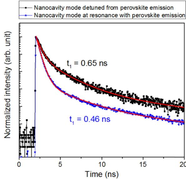
Fig. 5. Plot comparing the PL decay of the perovskite nanocrystals in two different cases: one which is coupled to the cavity (blue) and the other uncoupled (black) with the respective  $t_1$  decay time as labelled.
