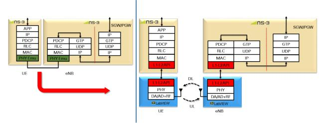
The ns-3 LTE module contains a PHY abstraction to emulate the different physical channels and does not include a full-fledged PHY layer implementation. This abstraction is replaced by a real-
