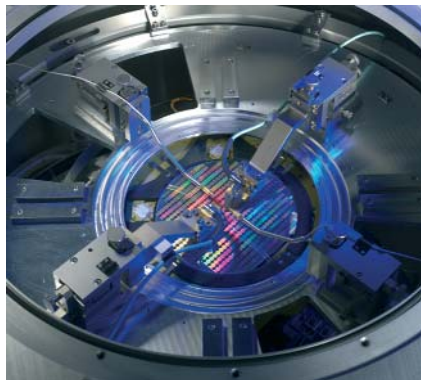
Figure 1: Test of pressure sensors (source: Süss MicroTec)
