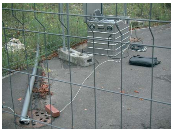
Figure 1: On-line odour measurements with OdourVector. The measurement system comprises a gas conditioning unit, a pre-concentration device, the measuring cell and a signal evaluation unit.
