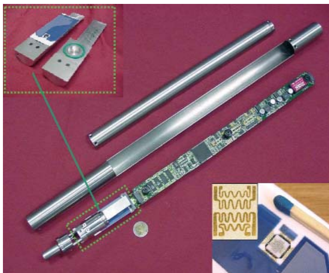
Figure: Battery operated tubular KAMINA module (diameter 32 mm, length 650 mm) for subsurface soil analysis integrated in electric hammer driven percussion probe, development funded by the Deutsche Bundesstiftung Umwelt (DBU, www.dbu.de ) (source: Forschungszentrum Karlsruhe GmbH)
