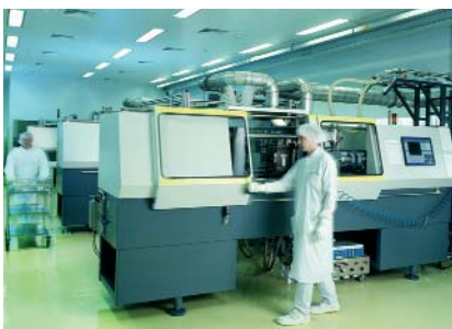
Figure 2: Injection moulding of microcomponents in a clean room (source: microParts)
