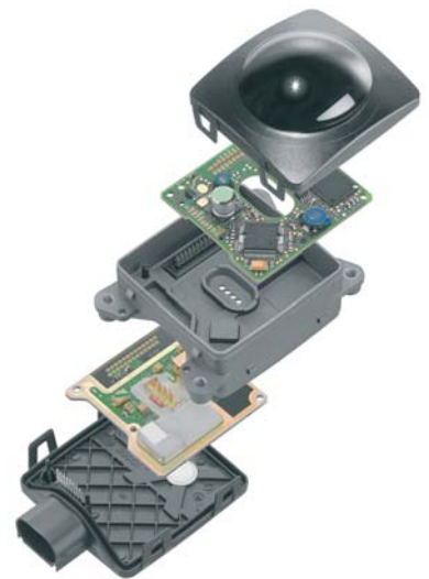
Figure 2: 77 GHz long-range Radar sensor with integrated CPU for Adaptive Cruise Control
