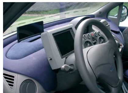
Figure 3: ICAR - HMI in the dash board and HMI - Prototype at the steering wheel
