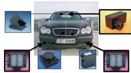
Figure 5: Test Vehicle with PMD camera, Illumination units, LDWS camera, Radar and IR ACC
