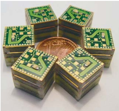
Figure 3: 3D stacking technology for self-organizing microsystems; (source: FhG-IZM, Berlin)
