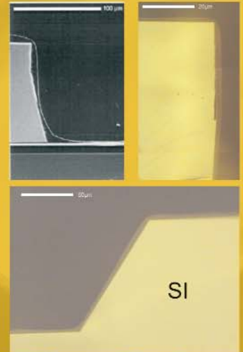
SEM Photographs of Spray Coated Cavities with Extreme Topography
